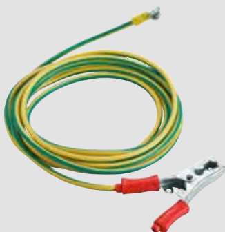
P/N KR4506 Earthing cable provided with plier. In environments with risk of explosion (i.e. with a potentially explosive atmosphere according to the ATEX directive) it is mandatory to connect to the ground both the pump and other equipment placed in the work area.
